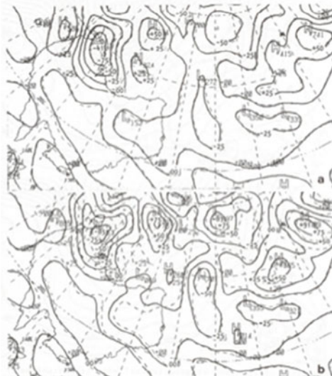
Fig. 9. Updated 500 mb vorticity when (a) weight on mass is zero, (b) weight on mass is 1000 poleward of 30°. The unprocessed analysis is dashed and the contour interval is 25 \cdot 10^{-6} \text{ sec}^{-1} .
